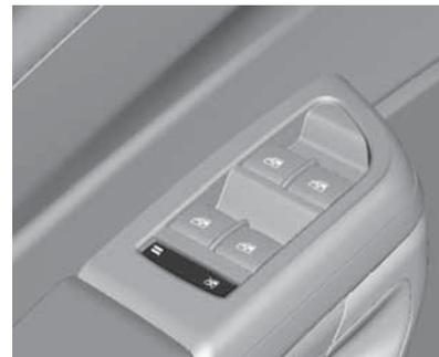
Pulse el interruptor
