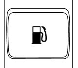
To open the fuel filler door, pull up on the release lever with this symbol on it. It is located on the floor on the outboard side of the driver's seat.
