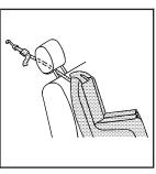
If the position you are using has an adjustable headrest or head restraint and you are using a single tether, route the tether under the headrest or head restraint and in between the headrest or head restraint posts.
