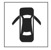
If one of the doors on the sedan is not closed properly while the ignition is on, the door ajar light on the instrument panel comes on and stays on until the doors are closed.
