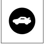
If your vehicle has a trunk release button located on the driver's door, you can open the trunk from inside your vehicle by pressing the release button.
