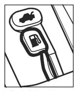
If your vehicle has a trunk release lever located on the outboard side of the driver's seat, you can open the trunk from inside your vehicle by pulling the release lever.
