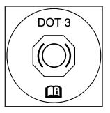
Your vehicle has one reservoir for both the brake and clutch hydraulic systems. It is filled with DOT-3 brake fluid. See Engine Compartment Overview on page 5-12 for the location of the reservoir.
