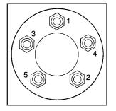
14. Tighten the wheel nuts firmly in a crisscross sequence, as shown, with the wheel wrench.
