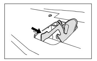
2. Then go to the front of the vehicle and push the secondary hood release handle toward the driver side of the vehicle.
