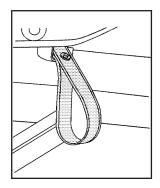
There is an assist handle located on the inside of the trunk.
