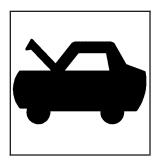
1. Pull the hood release handle with this symbol on it. It is located inside the vehicle to the left of the steering column.
