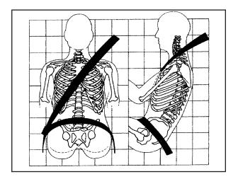
Sit up straight and always keep your feet on the floor in front of you. The lap part of the belt should be worn low and snug on the hips, just touching the thighs.
