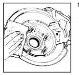
10. Remove any rust or dirt from the wheel bolts, mounting surfaces and spare wheel. 11. Install the compact spare tire.
