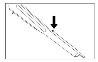
3. Extend the handle on the wheel wrench by pressing the button and pulling on the end of the wrench. You must do this before using the wheel wrench.
