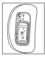
On vehicles with heated front seats, the buttons are located on the outboard side of the driver's and front passenger seats. Press the top of the switch again to go to the low heat setting. The indicator light will be lit next to the number 1.
