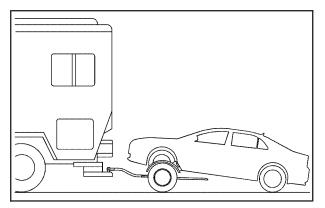
Tow the vehicle with the two rear wheels on the ground and the front wheels on a dolly:
