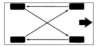
When rotating the vehicle's tires, always use the correct rotation pattern shown here.
