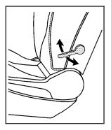
On vehicles with this feature, the handle is located on the outboard side of the seat.
