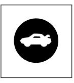
Press the button located on the driver door near the map pocket to open the trunk.
