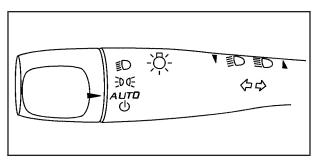
The band on the lever on the outboard side of the steering column operates the exterior lamps.
