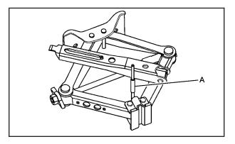
Place the jack over the bolt (A) on the floor, making sure it contacts the bolt. Thread the jack retainer nut until it contacts the jack.
