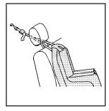
If the position you are using has an adjustable headrest or head restraint and you are using a dual tether route the tether under the headrest or head restraint and in between the headrest or head restraint posts. See *Head Restraints* on page 1-2.
