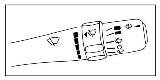
The windshield wiper lever is located on the right side of the steering wheel.
