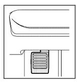
To set the parking brake, push down the parking brake pedal with your left foot. If the ignition is on, the brake system warning light will come on. See *Brake System Warning Light on page 3-34.*
