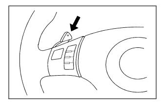
Press the + (plus) paddle located on top of the steering wheel controls forward to upshift, or push the backside of the shift paddle rearward to downshift.
