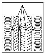
One way to tell when it is time for new tires is to check the treadwear indicators, which will appear when your tires have only 1/16 inch (1.6 mm) or less of tread remaining. You need new tires if any of the following statements are true:
