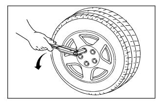
4. Use the wrench to loosen all the wheel nuts. Do not remove them yet.
