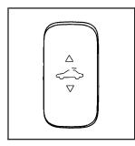
On vehicles with a sunroof, the switch is located on the headliner between the map lamps. The sunroof only operates when the ignition is in ON/RUN, ACC/ACCESSORY, or if Retained Accessory Power (RAP) is active. See *Retained Accessory Power (RAP) on page 2-23.*
