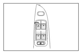
The power window switches are located on the armrest on the driver's door. In addition, there is a switch on each passenger door.
