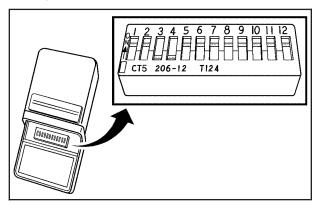
To verify that the garage door opener is a Fixed Code unit, remove the battery cover on the hand held transmitter supplied by the manufacturer of the garage door opener motor. If there are a row of dip switches similar to the graphic above, the garage door opener is a Fixed Code unit. If you do not see a row of dip switches, return to the previous section for Programming Universal Home Remote – Rolling Code.
