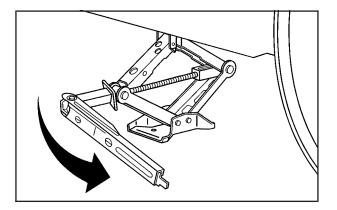
13. Lower the vehicle by turning the wrench counterclockwise. Lower the jack completely.
