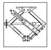
4. Raise the jack to the height shown and lock the wrench onto the jack.
