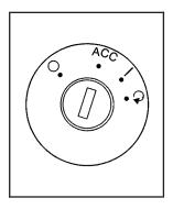
The ignition switch has four different positions.
