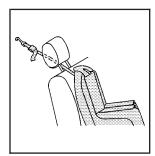
If the position you are using has an adjustable headrest or head restraint and you are using a single tether, route the tether under the headrest or head restraint and in between the headrest or head restraint posts. See *Head Restraints* on page 1-2. 3. Push and pull the child restraint in different directions to be sure it is secure.
