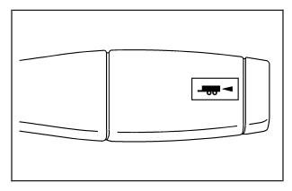
Your vehicle has a tow/haul mode. The button is located on the end of the column shift lever. Press the button to enable or disable the tow/haul mode. You can use this feature to assist when towing or hauling a heavy load. See "Tow/Haul Mode" under *Towing a Trailer on page 4-47* for more information.
