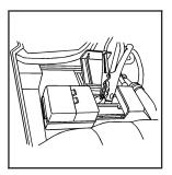
Connect the red positive (+) cable to the positive (+) terminal of the vehicle with the dead battery. Use a remote positive (+) terminal if the vehicle has one.
