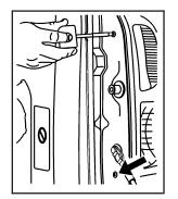
2. Remove the two screws from the taillamp assembly.
