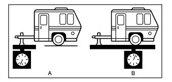
The trailer tongue weight (A) should be 10 percent to 15 percent of the total loaded trailer weight (B), up to a maximum of 600 lbs (272 kg) with a weight carrying hitch. The trailer tongue weight (A) should be 10 percent to 15 percent of the total loaded trailer weight (B), up to a maximum of 1,000 lbs (454 kg) for the 1500 series and up to a maximum of 1,500 lbs (680 kg) for the 2500 series with a weight distributing hitch.
