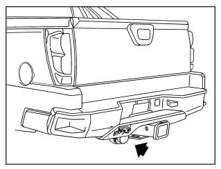
Your vehicle is equipped with the seven-wire trailer towing harness. This harness with a seven-pin universal heavy-duty trailer connector is attached to the rear bumper beam. It is located next to the integrated trailer hitch. The seven-wire harness contains the following trailer circuits:
