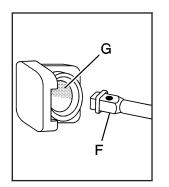
Insert the open end of the extension (F) through the hole in the rear bumper (G) (hoist shaft access hole).
