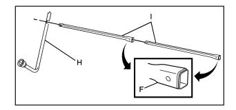
3. Assemble the two jack handle extensions (I) and wheel wrench (H) as shown.
