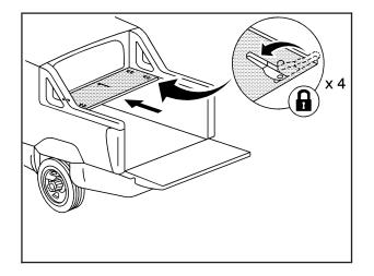
3. Push both left latches away from you to lock the latches. Remember that there are four latches total for panel 1. You should hear a click when each latch locks. Lock the remaining two right latches on panel 1.
