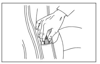
1. Remove the guide from its storage pocket on the side of the seatback.
