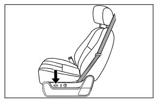
Driver's Seat with Power Seat Control, Power Recline, and Power Lumbar shown On a vehicle with power seats, the controls used to operate them are located on the outboard side of the seats. To adjust the seat, do any of the following:
