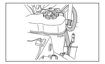
The coolant level should be at or above the FULL COLD mark. If it is not, you may have a leak at the pressure cap or in the radiator hoses, heater hoses, radiator, water pump or somewhere else in the cooling system.
