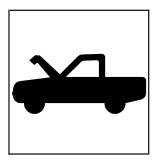
1. Pull the handle with this symbol on it. It is located inside the vehicle to the lower left of the steering wheel.
