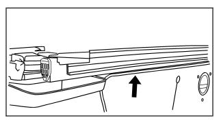
The side rail channels are located on top of both sides of the cargo area. Flush them out with clean water debris collects inside of them.
