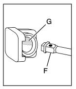
Insert the open end of the extension (F) through the hole in the rear bumper (G) (hoist shaft access hole).
