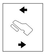
The switch used to adjust the pedals is located on the instrument panel below the climate control system. Press the arrow at the bottom of the switch to move the pedals closer to your body. Press the arrow at the top of the switch to move the pedals away from your body.
