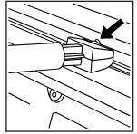
When placing the bows, locate the small notches in the side rails. These notches receive the tang on the bow ends and help the bows seat into place.
