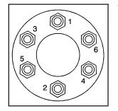
Tighten the nuts firmly in a crisscross sequence as shown by turning the wheel wrench clockwise.
