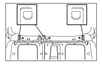
The top tether anchors are located on the back of the rear seat frame above the floor for each rear seating position. Fold down the rear seatback(s) to access the anchors. See *Rear Seat Operation on page 1-11*. Be sure to use an anchor located on the same side of the vehicle as the seating position where the child restraint will be placed.
