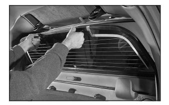
4. With the rear glass tilted at an angle, place the bottom edge in the lower channel of the window frame.
