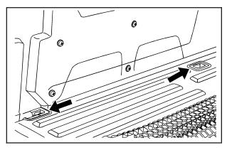
Your vehicle also has four cargo-area floor drains located under the cargo mat near the sides of the cargo area. These drains should be cleaned periodically to allow water to drain from the cargo area.
