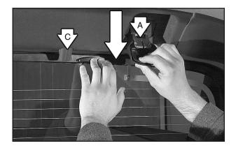
Squeeze and pull down the latch levers (A), located near the upper corners of the rear glass, to unlatch. Once unlatched, the glass-catch release button (C) will catch the rear glass and prevent it from falling forward.
