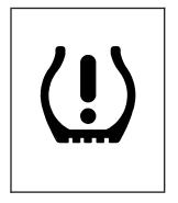
When a low tire pressure condition is detected, the TPMS illuminates the low tire pressure warning light located on the instrument panel cluster.
