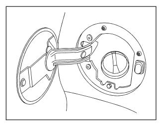
The tethered fuel cap is located behind a hinged fuel door on the driver's side of the vehicle. If the vehicle has E85 fuel capability, a yellow cap with the words "E85 or gasoline" can be seen.
