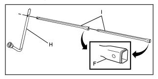
3. Assemble the two jack handle extensions (I) and wheel wrench (H) as shown.
