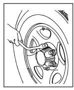
If the vehicle has a center cap, place the chiseled end of the wheel wrench in the slot on the wheel and gently pry the cap out.
