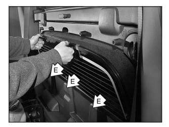
Load the rear glass into the storage pocket in the Midgate<sup>®</sup>, guiding the lower edge of the rear glass behind the three rear glass retaining tabs (E).
