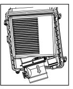
1. Locate the air cleaner/filter assembly. See Engine Compartment Overview on page 5-14.
