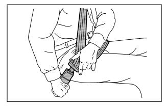
Push the latch plate into the buckle until it clicks. If you find that the latch plate will not go fully into the buckle, see if you are using the correct buckle. Pull up on the latch plate to make sure it is secure. If the belt is not long enough, see *Safety Belt Extender on page 1-33*. Make sure the release button on the buckle is positioned so you would be able to unbuckle the safety belt quickly if necessary.
