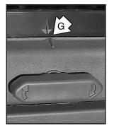
Be sure to align the rear glass side-to-side using the alignment arrows (G).
