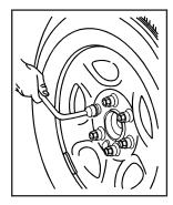
3. Use the wheel wrench to loosen all the wheel nuts. Turn the wheel wrench counterclockwise to loosen the wheel nuts. Do not remove the wheel nuts yet.
