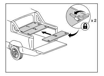
7. Push the latches away from you, starting with the left latch, to lock the panel in place. You should hear a click when each latch locks.
