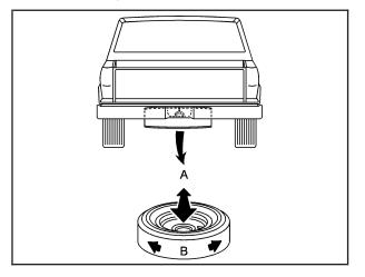
7. Make sure the tire is stored securely. Push, pull (A), and then try to turn (B) the tire. If the tire moves, use the wheel wrench to tighten the cable.
