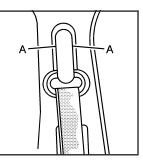
To move it down, squeeze the buttons (A) on the sides of the height adjuster and move the height adjuster to the desired position.
