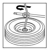
Use the wheel wrench hook that allows you to pull the hoist cable towards you, to assist in reaching the spare tire.
