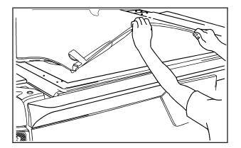
2. Pull the back of the cover out from the rear rail (D).
