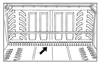
The Midgate<sup>®</sup> drain grate is located near the base of the Midgate<sup>®</sup> in the cargo area. You will find a removable drain grate covering the drain.
