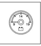
When your engine is not running, but the ignition is on, this gage shows the battery's state of charge in DC volts.
