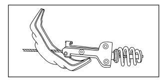
2. Tilt the tire. Separate the tire/wheel retainer (D) from the guide pin. Pull the pin through the center of the wheel. Tilt the retainer down through the center wheel opening.
