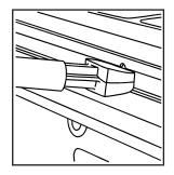
2. Remove the two bows by gently pushing them against the spring-loaded end. Set the bow aside.
