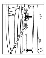
2. Remove the two rear lamp assembly screws near the tailgate latch.
