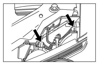
2. Reach in to access either one of the bulb sockets in the engine compartment.
