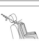
If the position you are using has an adjustable headrest or head restraint and you are using a single tether, raise the headrest or head restraint and route the tether under the headrest or head restraint and in between the headrest or head restraint posts.
