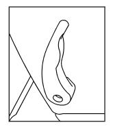
To fold the seatback forward, push the lever on the side of the seat rearward and pull the seatback forward.
