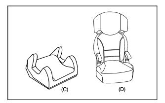
A booster seat (C-D) is a child restraint designed to improve the fit of the vehicle's safety belt system. A booster seat can also help a child to see out the window.
