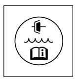
The hydraulic clutch fluid reservoir cap has this symbol on it. See *Engine Compartment Overview on page 5-12* for reservoir location.
