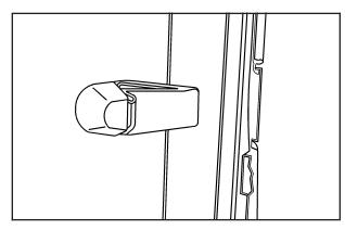
If your vehicle has this feature, squeeze the latch in the center of the window and slide the glass to open it.
