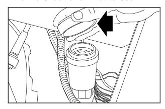
Refer to the Maintenance Schedule to determine how often you should check the fluid level in your clutch master cylinder reservoir and for the proper fluid. See *Recommended Fluids and Lubricants on page 6-12*.
