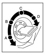
With the key in the ignition switch, you can turn to four different positions.
