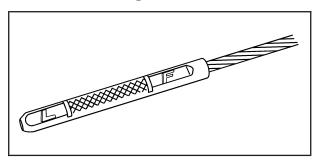
If the oil is below the cross-hatched area (L), add at least one quart/liter of the recommended oil. This section explains what kind of oil to use. For engine oil crankcase capacity, see *Capacities and Specifications* on page 5-120.
