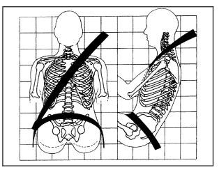
Sit up straight and always keep your feet on the floor in front of you. The lap part of the belt should be worn low and snug on the hips, just touching the thighs. In a crash, this applies force to the strong pelvic bones and you would be less likely to slide under the lap belt. If you slid under it, the belt would apply force on your abdomen. This could cause serious or even fatal injuries.
