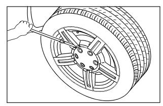
Remove the center cap by placing the chisel end of the wheel wrench (E) into one of the slots on the wheel and gently prying the cap out.
