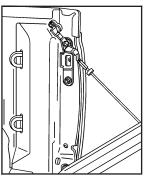
2. Remove the retaining cable from the passenger side of the tailgate by pulling the clip away from the bolt head while pushing the cable bracket forward.
