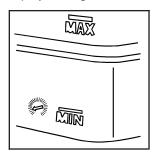
The fluid level should be above MIN. If it is not, have the brake hydraulic system checked to see if there is a leak.
