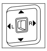
If your vehicle has this feature, the controls are located on the driver's door armrest.
