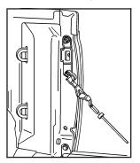
Remove the retaining cables from both sides of the tailgate by pulling the clips away from the bolt heads while pushing the cable bracket forward. When the larger part of the hole on the bracket is over the bolt, slide the bracket off of the bolt.
