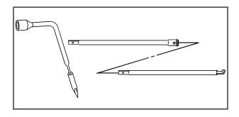
3. Attach the wheel wrench and extensions together as shown.
