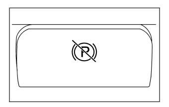
To release the parking brake, hold the regular brake pedal down. Pull the bottom edge of the lever, located above the parking brake pedal, with the parking brake symbol, directly rearward to release the parking brake. If the ignition is on when the parking brake is released, the brake system warning light will go off.
