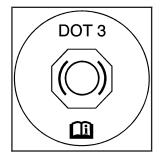
The brake master cylinder reservoir is filled with DOT-3 brake fluid. See *Engine Compartment Overview on page 5-12* for the location of the reservoir.
