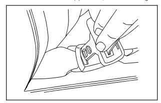
Disconnect the rear center safety belt latch from the mini buckle by inserting the tip of the safety belt tongue into the slot on the buckle. Let the belt retract.
