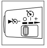
The cruise control set button is located at the end of the multifunction lever.
