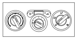
The heating, cooling, and ventilation for your vehicle can be controlled with this system.
