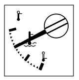
This gage shows the engine coolant temperature.
