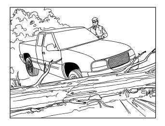
If your vehicle stalls when you are crossing an incline, be sure you, and any passengers, get out on the uphill side, even if the door there is harder to open. If you get out on the downhill side and the vehicle starts to roll over, you will be right in its path.
