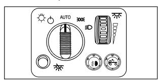
The control on the driver's side of the instrument panel operates the exterior lamps.
