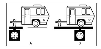
The trailer tongue weight (A) should be 10 percent to 15 percent of the total loaded trailer weight, up to a maximum of 500 lbs (226 kg) with a weight carrying hitch.
