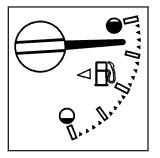
When the ignition is on, the fuel gage shows how much fuel the vehicle has remaining in the fuel tank.
