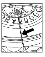
Check under the vehicle to see if the cable end fitting is visible.
