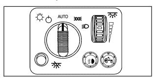
The exterior lamp control is located on the instrument panel on the left side of the steering wheel.
