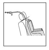
If the position you are using has a fixed headrest or head restraint and you are using a single tether, route the tether over the head restraint.
