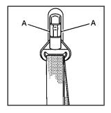
To move it up or down, squeeze the release buttons (A) together and move the height adjuster to the desired position.
