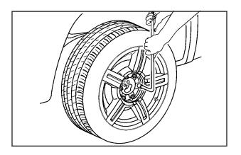
Use the wheel wrench to loosen all the wheel nuts by turning it counterclockwise. Do not remove the wheel nuts yet.
