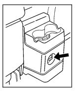
Put the cover in position and insert and tighten the wing nut to secure it.
