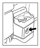
Turn the wing nut on the cover counterclockwise to remove it.
