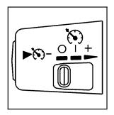
These controls are located at the end of the multifunction lever.
