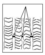
One way to tell when it is time for new tires is to check the treadwear indicators, which appear when your tires have only 1/16 inch (1.6 mm) or less of tread remaining. Some commercial truck tires may not have treadwear indicators.
