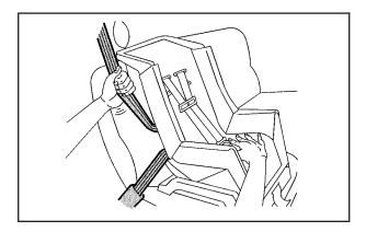
6. To tighten the belt, push down on the child restraint, pull the shoulder portion of the belt to tighten the lap portion of the belt, and feed the shoulder belt back into the retractor. If you are using a forward-facing child restraint, you may find it helpful to use your knee to push down on the child restraint as you tighten the belt.
