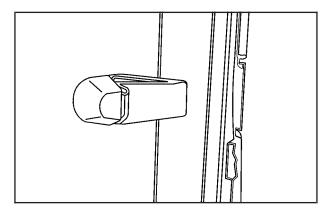
If the vehicle has this feature, squeeze the latch in the center of the window and slide the glass to open it.
