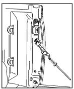
Remove the retaining cables from both sides of the tailgate by pulling the clips away from the bolt heads while pushing the cable bracket forward.
