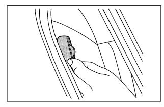
Slide the guide off of its storage clip located between the interior body and the seatback.
