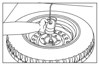
Tilt the retainer downward and through the center wheel opening. Make sure the retainer is fully seated across the underside of the wheel.
