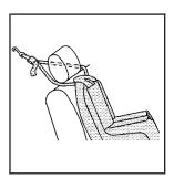
If the position you are using has a fixed or adjustable headrest or head restraint and you are using a dual tether, route the tether around the headrest or head restraint.
