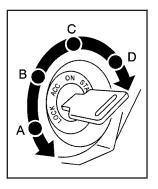
The ignition switch has four different positions.
