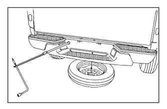
Insert the chiseled end of the jack handle at a slight angle through the hole in the rear bumper and into the funnel-shaped guide.
