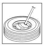
Tilt the retainer when the tire has been lowered, and slide it up the cable so it can be pulled up through the wheel opening.
