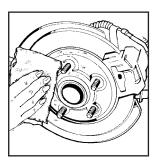
Remove any rust or dirt from the wheel bolts, mounting surfaces and spare wheel. 9. Install the spare tire.
