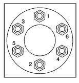
Tighten the wheel nuts firmly in a crisscross sequence as shown by turning the wheel wrench clockwise.
