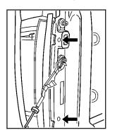
2. Remove the two rear lamp assembly screws near the tailgate latch.
