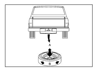
7. Make sure the tire is stored securely. Push, pull (A), and then try to turn (B) the tire. If the tire moves, check to make sure the tire valve stem is pointing down, then use the wheel wrench to loosen and then tighten the cable.
