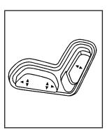
If the seats have power reclining seatbacks, use the vertical power seat control located on the outboard side of the seat.
