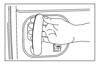
To open the sliding side door from the inside, turn the handle upward and toward the rear of the vehicle. Then, slide the door toward the rear of the vehicle.
