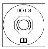
The brake master cylinder reservoir is filled with DOT-3 brake fluid. See Engine Compartment Overview on page 5-14 for the location of the reservoir.
