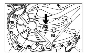
If the level is below the bottom of the filler plug hole, you'll need to add some lubricant. Add enough lubricant to raise the level to the bottom of the filler plug hole. Use care not to overtighten the plug.
