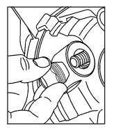
Put the wheel nuts back on with the rounded end of the nuts toward the wheel. Tighten each wheel nut by hand until the wheel is held against the hub.
