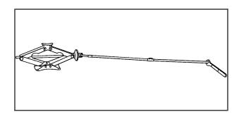
Attach the jack handle/jack handle extension to the jack. With the UP mark facing you, slide the ratchet onto the end of the jack handle extension.
