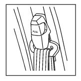
To move it down, pull on the center adjuster control labeled PULL. You can move the height adjuster up just by pushing up on the shoulder belt guide.
