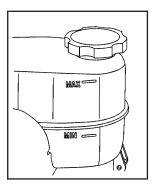
The fluid level should be above MIN. If it is not. have the brake hydraulic system checked to see if there is a leak.
