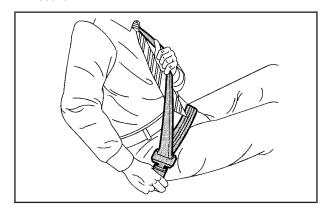
To make the lap part tight, pull up on the shoulder belt. It may be necessary to pull stitching on the safety belt through the latch plate to fully tighten the lap belt on smaller occupants.
