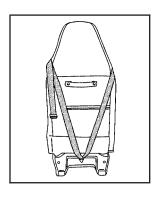
If the position you are using has an integrated headrest or head restraint and you are using a dual tether, route the tether around the headrest or head restraint.
