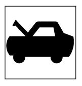
Pull the handle with this symbol on it. It is located in front of the driver's side door frame near the floor.
