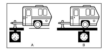
The trailer tongue weight (A) should be 10 percent to 15 percent of the total loaded trailer weight (B), up to a maximum of 400 lbs (181 kg) with a weight carrying hitch. The trailer tongue weight (A) should be 10 percent to 15 percent of the total loaded trailer weight (B), up to a maximum of 1,000 lbs (454 kg) with a weight distributing hitch.
