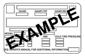
A vehicle specific Certification/Tire label is found on the rear edge of the driver's door. The label shows the size of your vehicle's original tires and the inflation pressures needed to obtain the gross weight capacity of your vehicle. This is called Gross Vehicle Weight Rating (GVWR). The GVWR includes the weight of the vehicle, all occupants, fuel, and cargo.
