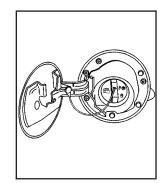
The tethered fuel cap is located behind a hinged fuel door on the driver side of the vehicle.
