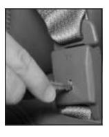
To do this, press the tip of a key into the release hole of the safety belt buckle while pulling up on the safety belt.
