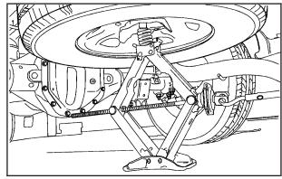
Place the jack under the vehicle, ahead of the rear bumper. Position the center lift point of the jack under the center of the spare tire and turn the handle clockwise to raise the jack until it lifts the secondary latch spring.
