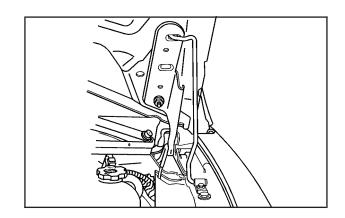
Lift the hood, release the hood prop from its retainer and put the hood prop into the slot in the hood.
