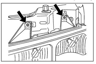
Remove the two pins on the top of the headlamp assembly. To remove the pins, turn the outer pin clockwise and pull it straight up. To remove the inner pin, turn it counterclockwise and pull it straight up.
