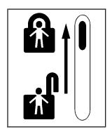
For the side sliding door, move the button up to engage the security feature. Move the button down to return the door locks to normal operation.
