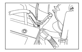
Connect the red positive (+) cable to the positive (+) terminal of the dead battery. Use a remote positive (+) terminal if the vehicle has one.
