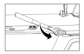
Turn the ratchet counterclockwise to lower the spare tire to the ground. If the spare tire does not lower to the ground, the secondary latch is engaged causing the tire not to lower. See Secondary Latch System on page 5-93.
