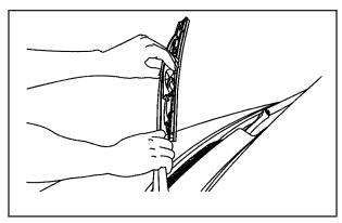
Press down on the blade assembly pivot locking tab. Pull down on the blade assembly to release it from the wiper arm hook.
