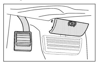
To set the parking brake, hold the regular brake pedal down with your right foot. Push down the parking brake pedal with your left foot.
