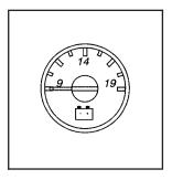
When your engine is not running, but the ignition is on, this gage shows the battery's state of charge in DC volts.
