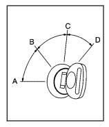
Use the key to turn the ignition switch to four different positions.
