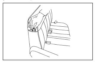
Locate the guide in a pocket on the side of the seatback.
