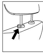
Pull the head restraint up to raise it. To lower the head restraint, press the button, located on the top of the seatback, and push the restraint down. Only the front head restraints are adjustable.
