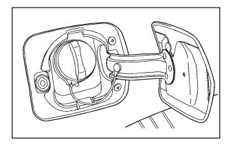
The tethered fuel cap is located behind a hinged fuel door on the passenger side of the vehicle. If the vehicle has E85 fuel capability, the fuel cap will be yellow and state that E85 or gasoline can be used. See *Fuel E85 (85% Ethanol) on page 5-7*.
