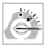
The fuel gage indicates about how much fuel is left in the fuel tank.
