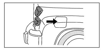
To open the fuel door, push the rearward center edge in and release and it will open.
