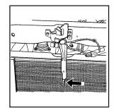
2. Then go to the front of the vehicle and push the secondary hood release lever to the left. It is located under the front center of the grille.
