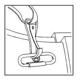
9. Attach the strap to the cargo tie-downs in the rear of the vehicle.
