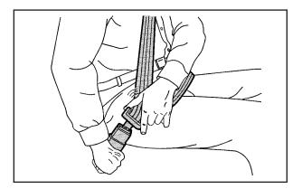
3. Push the latch plate into the buckle until it clicks. Pull up on the latch plate to make sure it is secure. If the belt is not long enough, see *Safety Belt Extender on page 1-31*.
