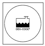
The coolant recovery tank cap has this symbol on it. The tank is located in the engine compartment toward the front of the engine on the passenger's side of the vehicle.
