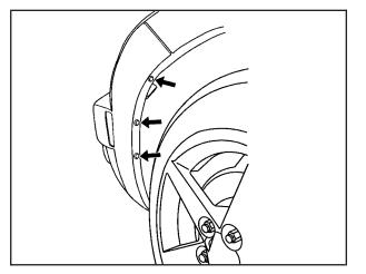
2. Remove the fasteners located on the wheel liner. To access the headlamp and the turn signal/parking lamp bulbs.
