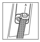
Push down on the release button (A) and move the height adjuster to the desired position. The adjuster can be moved up by pushing the release button up on the shoulder belt guide.
