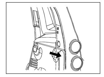
The vehicle may have a power plug connector located in the rear cargo area on the passenger side behind the service panel. The power connector wiring can be accessed by removing the service panel to begin installation. This plug can be used to supply power to commercial converters and contains four different circuits. The functions of these circuits are as follows; a 40 Amp battery service, a 10 Amp Accessory or Run service, a 15 Amp Delayed Accessory service and a Ground circuit.
