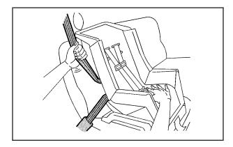
5. To tighten the belt, push down on the child restraint, pull the shoulder portion of the belt to tighten the lap portion of the belt and feed the shoulder belt back into the retractor. When installing a forward-facing child restraint, it may be helpful to use your knee to push down on the child restraint as you tighten the belt.
