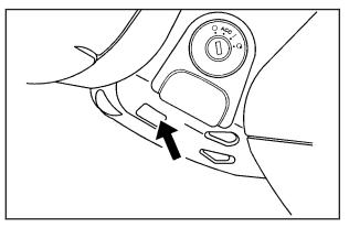
2. Remove the cover from the bottom of the steering column.
