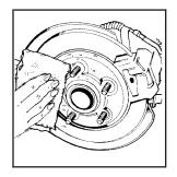
7. Remove any rust or dirt from the wheel bolts, mounting surfaces, and wheel.
