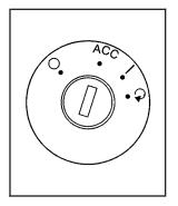
The ignition switch has four different positions.
