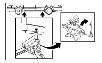
3. Position the jack on the rear position and raise the jack lift head to fit over the car flange under the down arrow markings on the rocker panel.
