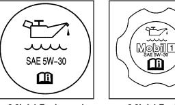
2.2L L4 Engine and 2.4L L4 Engine 2.0L L4 Engine
