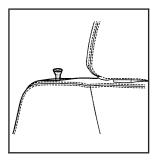
Pull up on the knob located on the top of the seatback on the outboard side to release the seatback.
