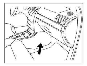
The floor console fuse block is located on the passenger side of the floor console behind the forward panel. The panel has four clips, one in each corner. Pull the panel to disconnect the four clips, and access the fuses. Use the fuse puller to remove fuses.
