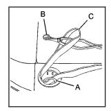
Route the loop end of the strap (C) through one of the cargo tie-downs (A) located in the rear of the vehicle.
