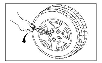
2. Using the wheel wrench, loosen all the wheel nuts on the rear tire. Do not remove them yet.
