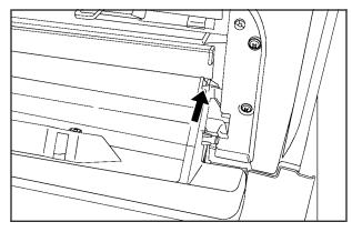
2. Press both glove box stops outward to let the glove box drop open completely.
