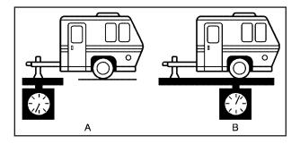
If using a weight-carrying hitch, the trailer tongue (A) should weigh 10 to 15 percent of the total loaded trailer weight (B).
