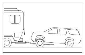
Use the following procedure to dolly tow the vehicle from the front with two wheels on the ground:
