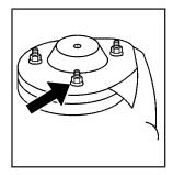
Locate the remote negative (–) ground terminal, marked GND (–), which is located at the front of the engine compartment on the driver side of the vehicle.
