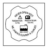
1. Remove the pressure cap when the cooling system, including the pressure cap and upper radiator hose, is no longer hot.
