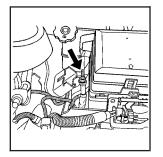
Locate the remote positive terminal which is located under a red tethered cap on the engine compartment fuse block. Remove the cap to access the terminal.
