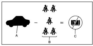
Refer to your vehicle's tire and loading information label for specific information about your vehicle's maximum vehicle capacity weight and seating positions. The combined weight of the driver, passengers, and cargo should never exceed your vehicle's maximum vehicle capacity weight.
