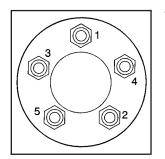
10. Tighten the wheel nuts firmly in a crisscross sequence as shown.
