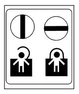
On vehicles with this feature, the rear door security locks are located on the inside edge of each rear door. You must open the rear doors to access them. To open a rear door while the security lock is on, do the following:
