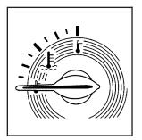
The vehicle has an engine coolant temperature gage. With the ignition turned to ON/RUN, this gage shows the engine coolant temperature.
