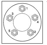
11. Tighten the wheel nuts firmly in a crisscross sequence, as shown.
