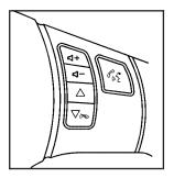
Vehicles with audio steering wheel controls could differ depending on the vehicle's options. Some audio controls can be adjusted at the steering wheel.  $\triangleleft$  + /  $\triangleleft$  – (Volume): Press to increase or to decrease the radio volume.
