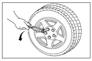
2. Using the wheel wrench, loosen all the wheel nuts. Do not remove them yet.
