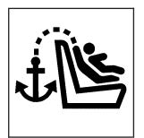
To assist you in locating the top tether anchors, this symbol will be located on the lower side quarter panels for the rear outboard positions, on the storage compartment for the rear center position and on the cargo mat behind the rear seats.
